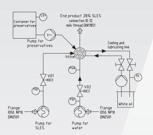
Main component of the system is a three stage Inline dispersing and homogenising machine. Additional to the normal axial inlet this machine is equipped with two or three additional radial inlets directly into the dispersing chambers for additional dosing of components.
